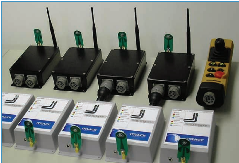
Figure 4: Local positioning and tracking system, or LPTS
